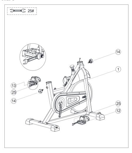
Install the right pedal (12) with R mark on The Main Body (1) and fix it with an open wrench (25). Note: tighten it clockwise.
