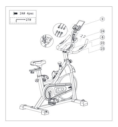
First put the electronic watch (9) on the electronic watch fixing plate of the armrest (6), pass the induction wire through the round hole in the middle of the fixing plate, and install the electronic watch on the fixing plate with screws (24);
