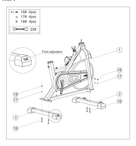
The Front Stabilize (2) is fixed on the Main Body (1) with Carriage Bolts (16), Flat washers (17) and cover nuts (18), and fixed with open wrench (25). Note: the move wheels of the Front Stabilize(2) are forward, as shown.
