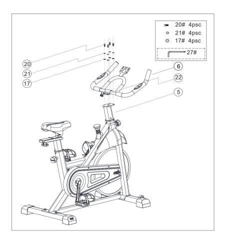
The Handle Frame (6) is fixed on the Handle Post (5) with Flat washers (17), the Spring washers (21) and the Button head bolts (20), and tightened with an inner hexagonal wrench (27).
