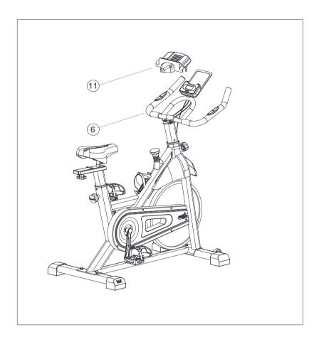
Install the Mobile phone holder (11) on the Handle Frame (6).
