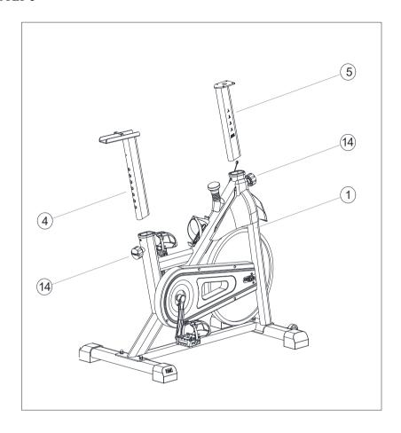
The Saddle Post (4) is inserted into the Main Body (1), and the Adjusting knob (14) is pulled out so that the Adjusting knob (14) is automatically inserted into the corresponding hole of the Saddle Post (4).
